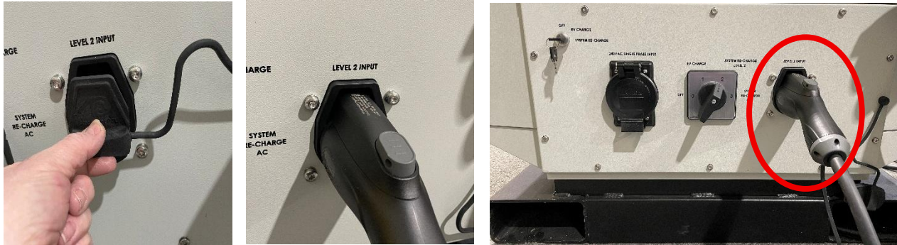
Figure 12—Level 2 Inlet cover being removed and Level 2 EV charger's output cable handle plugged into EVPC3082 Charger's Level 2 Inlet
