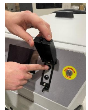
Figure 30—After entering Configuration Mode, pressing top or bottom button will increase or decrease maximum power setting
