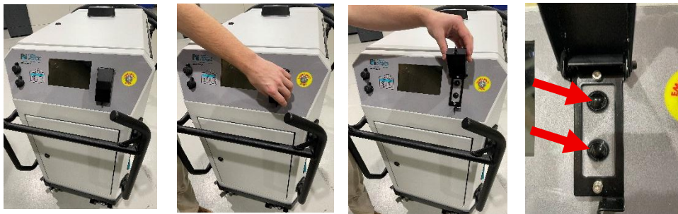
Figure 28—Lift button cover and press top and bottom buttons simultaneously to enter Configuration Mode
