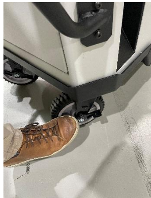
Figure 4.1—Unlocking wheel and Lock Lever in OFF position
