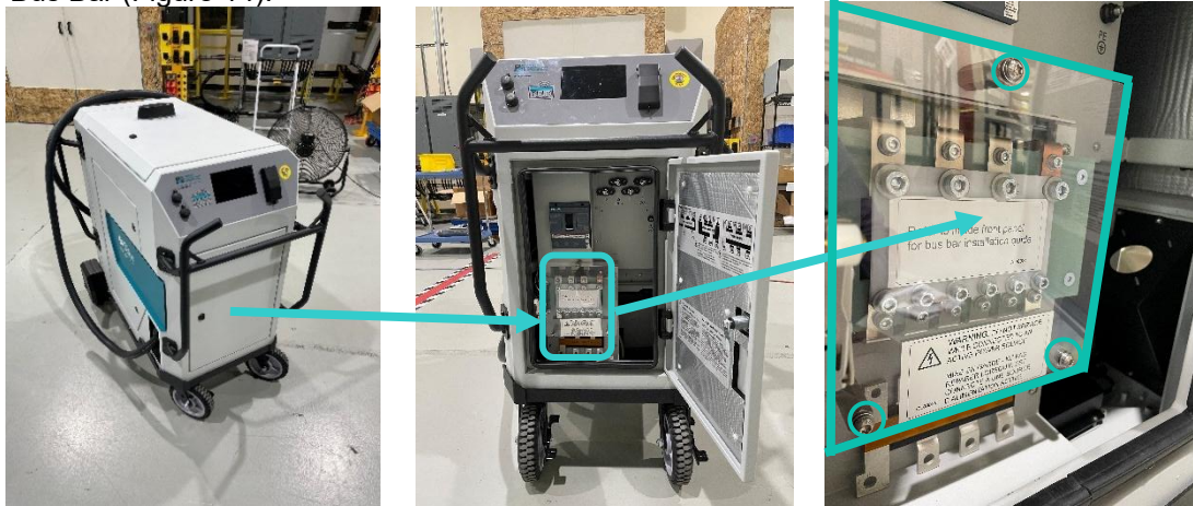
Figure 14—Open front door to locate clear, protective plate anchored in front of Bus Bar
