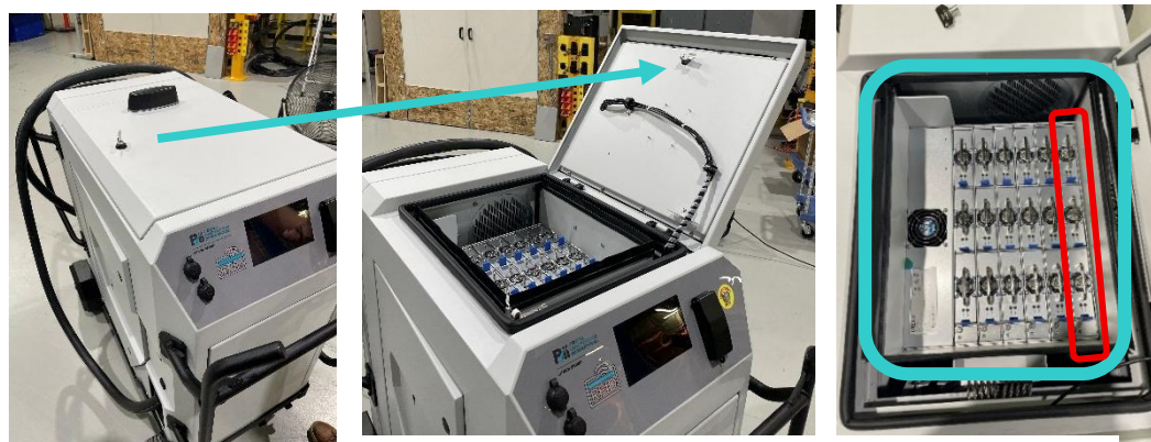
Figure 6—From front of charger, Top Door will open to the right side of charger; Red highlight indicates the "bottom" shelf of power stack.
