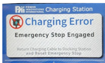
Figure 32—Error Message displays in LCD screen when Emergency Stop Button is depressed
