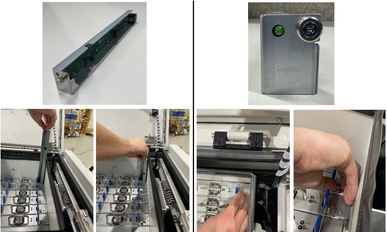
Figure 9—Installing Shelf Controller in top SC slot
