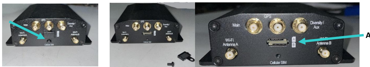
Figure 25 – For Peplink Modem, remove 1 screw and small slot cover to expose SIM card slots A and B
