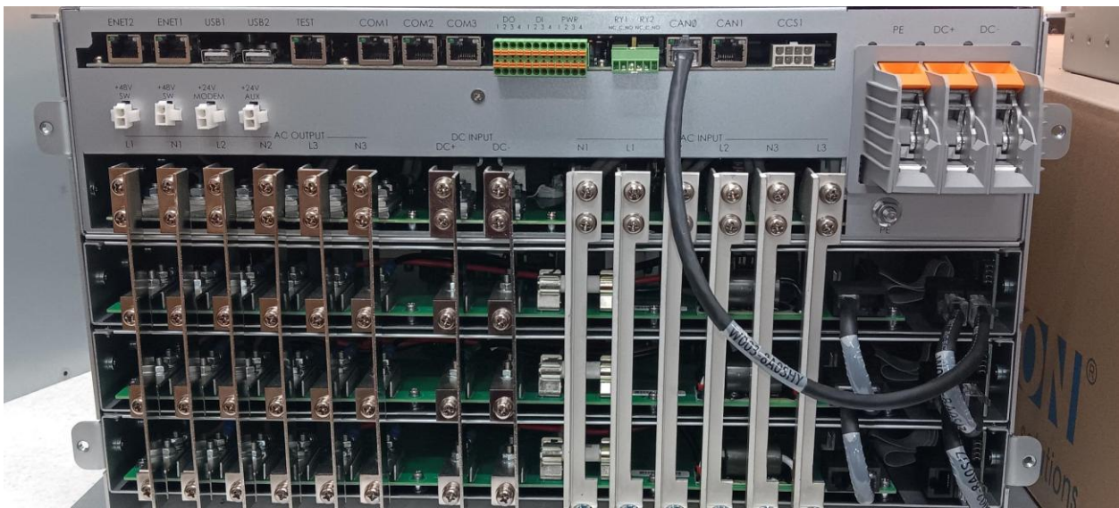
Figure 6 –Rack Controller installed in a power stack
