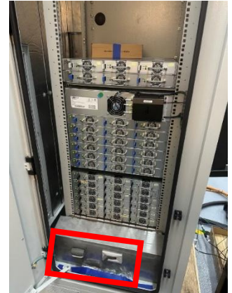
Figure 2 – Main Switch and its removeable handle shown in a fully loaded 60kW Bi-Directional Charger (inside left-side door)
