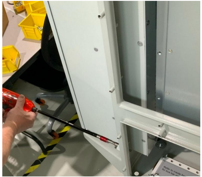
Figure 9 – Removing 20 fasteners from each heat exchanger (HX) (left-side HX and right-side HX)
