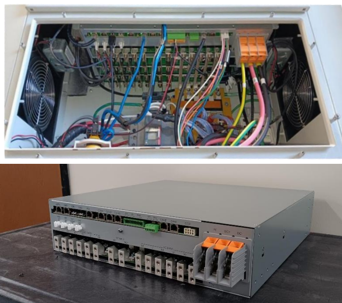
Figure 1: Rack controller (above) as installed and wired in a 30 kW EV quick charger and (below) when uninstalled
