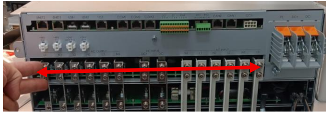
Figure 7 – The 28 bus screws (or 2 rows of 14 screws) closest to the front of the charger must be removed before rack controller can be pulled from charger
