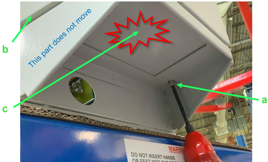
Figure 8 – Removing Heat Exchangers from both sides of the charger
