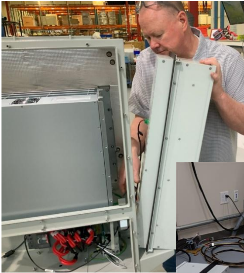
Figure 10 – Removing Heat Exchangers from both sides of the charger
