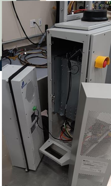
Figure 9 – Removing 20 fasteners from each heat exchanger (HX) (left-side HX and right-side HX)
