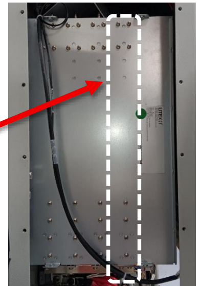
Figure 11 – Eight forward screws on each side of the charger are accessible once HX covers are removed
