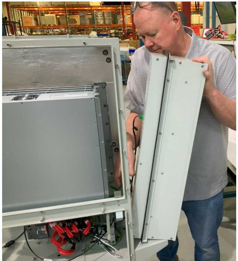
Figure 9 – Removing heat exchanger
