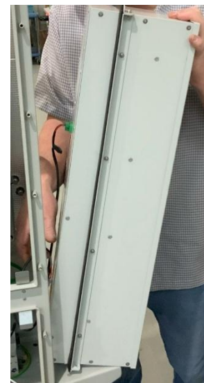
Figure 12 – Remove heat exchanger from back of charger PLACEHOLDER
