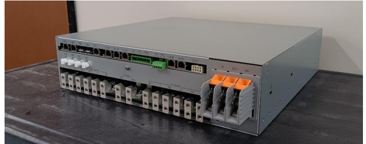
Figure 18 – Back of uninstalled Rack Controller
