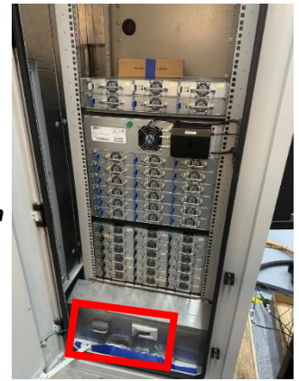
Figure 4 – Main Switch and its removeable handle shown in a fully loaded 60kW Bi-Directional Charger (inside left-side door)
