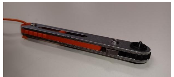
Figure 12 –Ratcheting right-angle screwdriver
