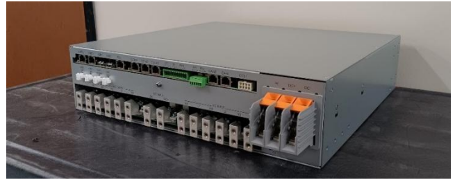
Figure 14 – Rack Controller back with Top Cover on
