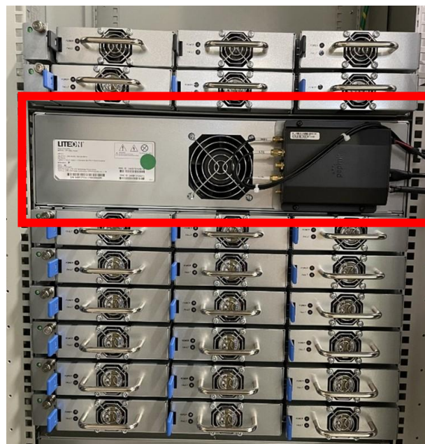
Figure 1: Rack Controller (highlighted) mounted in this 60 kW Bi-Directional Charger's power stack
