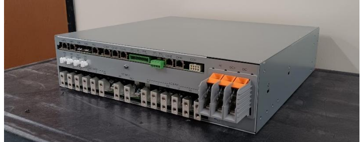
Figure 14 – Back of uninstalled Rack Controller
