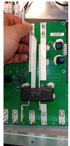
Figure 19 – L-shaped Relay busbars and DC busbars being removed
