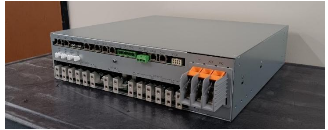
Figure 14 – Rack Controller, back view with Top Cover on
