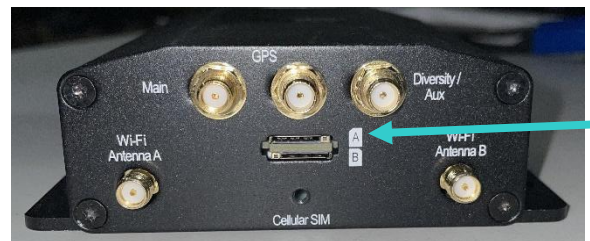
Figure 36 - Removing screw and small slot cover to expose SIM card slots A and B
