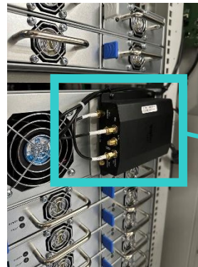
Figure 35 - Locating pre-installed cellular modem inside left-side door
