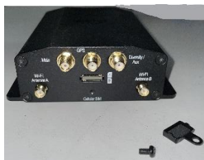
Figure 35 - Removing screw and small slot cover to expose SIM card slots A and B
