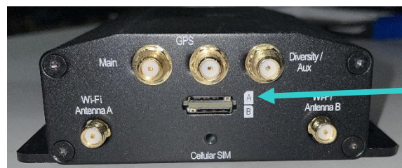
Figure 35 - Removing screw and small slot cover to expose SIM card slots A and B
