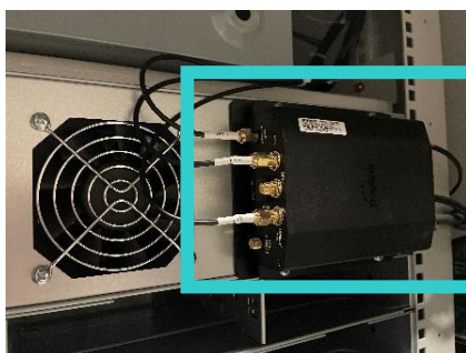
Figure 34 - Locating pre-installed cellular modem inside left-side door
