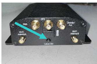
Figure 35 - Removing screw and small slot cover to expose SIM card slots A and B
