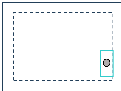
Figure 8 - AC power-in cables routed out of concrete within charger’s footprint marks on ground
