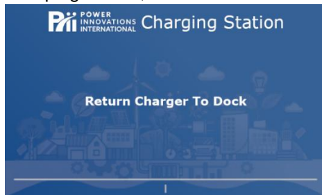
When Cable is unplugged from EV
