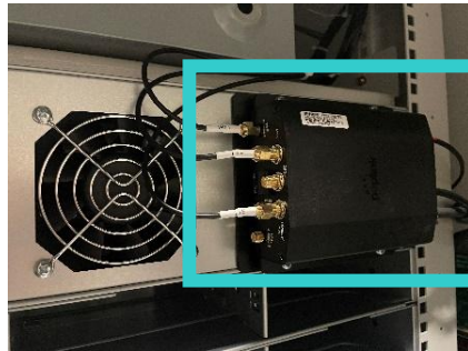
Figure 35 - Locating pre-installed cellular modem inside left-side door
