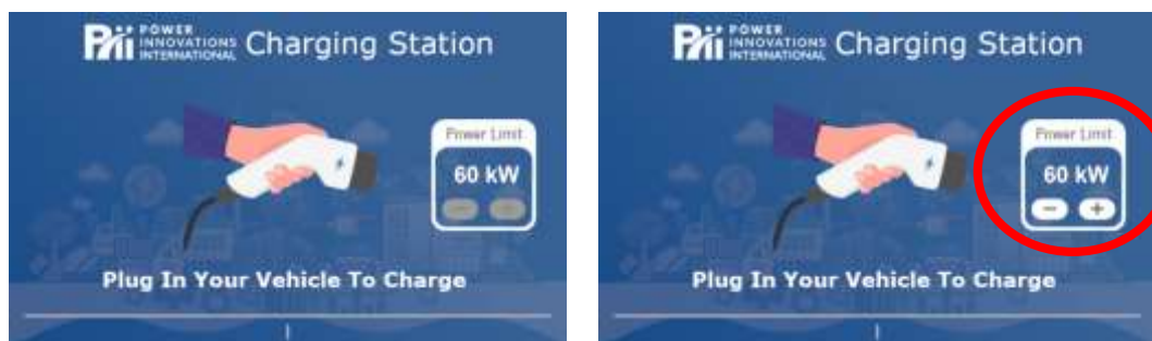
Figure 25—On-screen display of Maximum Power Level – and + buttons will brighten when charger enters Configuration Mode
