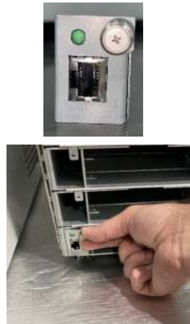
Figure 8—Secure Shelf Controllers
