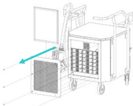
Figure 5—Optional Removal of Screen
