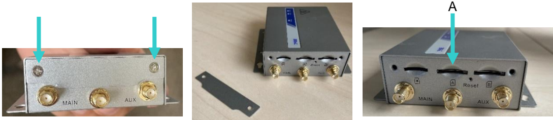
Figure 11— For Amit Modem, remove 2 screws and slot cover to expose SIM card slots
