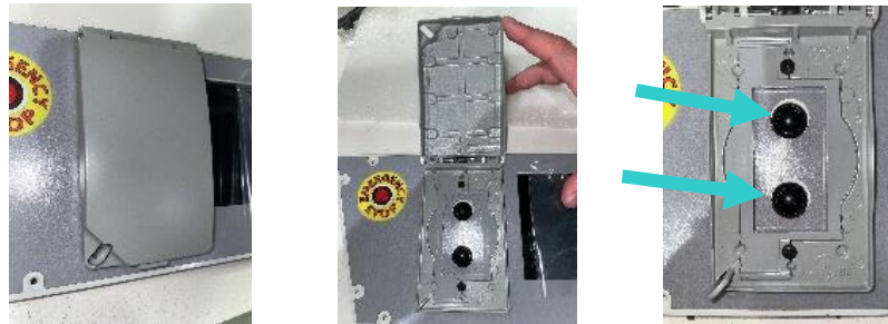
Figure 24—Lift button cover and press top and bottom button simultaneously to enter Configuration Mode
