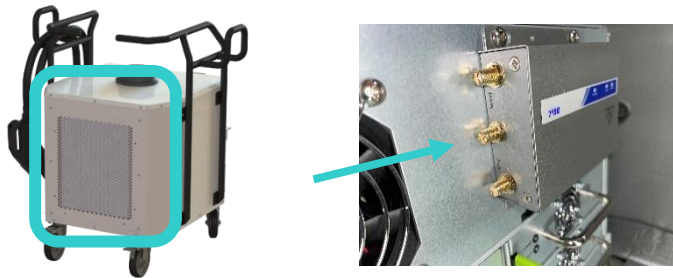
Figure 10—Remove Rear Cover to access cellular modem
