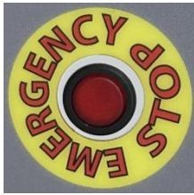
Figure 27—Emergency Stop Button is ON/OFF operator button: Recessed is OFF and Flush is ON
