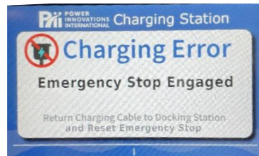
Figure 28—Error Message displays in LCD screen when Emergency Stop Button is depressed
