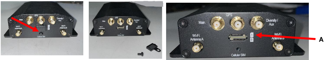
Figure 21 – For Peplink Modem, remove 1 screw and small slot cover to expose SIM card slots A and B
