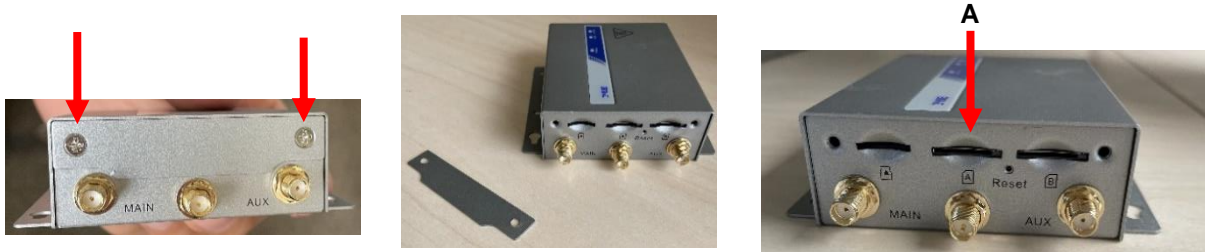
Figure 20 – For Amit Modem, remove 2 screws and slot cover to expose SIM card slots
