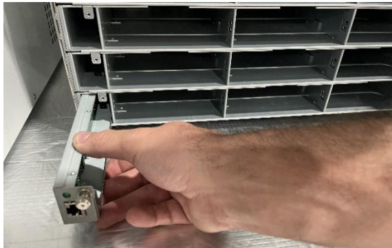
Figure 17.1 – Install Shelf Controllers
