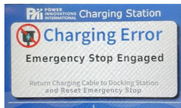
Figure 29—Error Message displays in LCD screen when Emergency Stop Button is pushed
