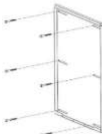
Figure 8—Lag screws and flat washers with hanging bracket
