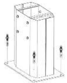
Figure 11—Anchor Pedestal to concrete
