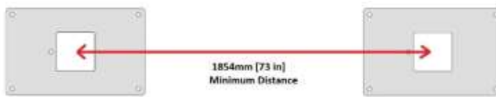
Figure 6—Minimum space between pedestal baseplate is 73 inches (1854 mm)
