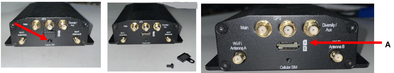
Figure 27 – For Peplink Modem, remove 1 screw and small slot cover to expose SIM card slots A and B
