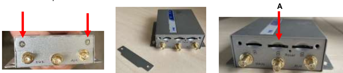
Figure 26 – For Amit Modem, remove 2 screws and slot cover to expose SIM card slots
