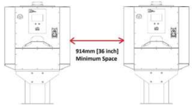
Figure 3—Minimum space between mounted chargers should be 36 in. (914 mm)
