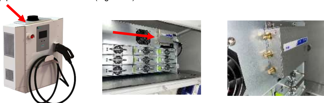
Figure 25—Remove Top Panel to access cellular modem
