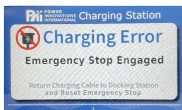
Figure 34—Error Message displays in LCD screen when Emergency Stop Button is pushed
