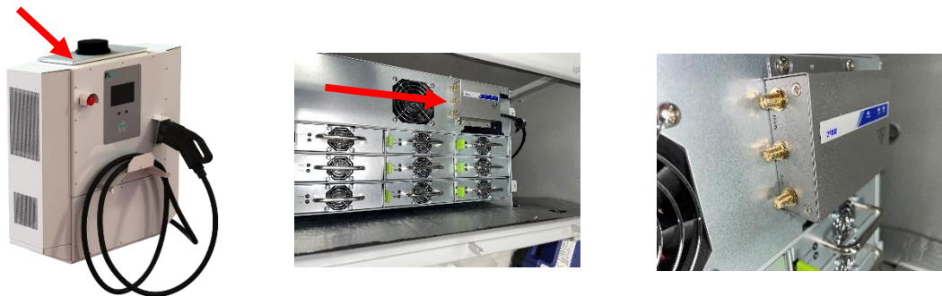
Figure 25—Remove Top Panel to access cellular modem
