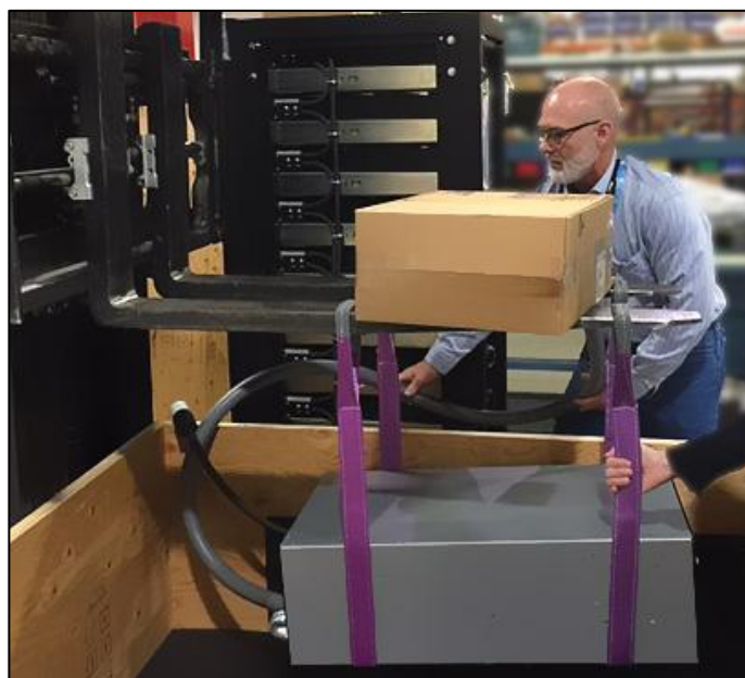
Figure 2—Chameleon 100 Being Lowered Using the Webbing Sling and Forklift
