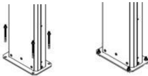
Figure C: Pedestal with Wedge Anchors before and after installation
